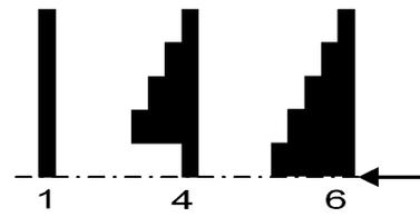
Fig. 5. Simplified slab structure (type of hardness profile) most frequently found in Swiss and Canadian data sets ( $N = 186$ ). Frequency of profile types 1: 36%, 4: 7.5%, 6: 38%.
