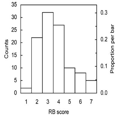
Fig. 2. Rutschblock scores of RB tests adjacent to human triggered slab avalanches. Swiss and Canadian cases shown together ( $N = 106$ ).
